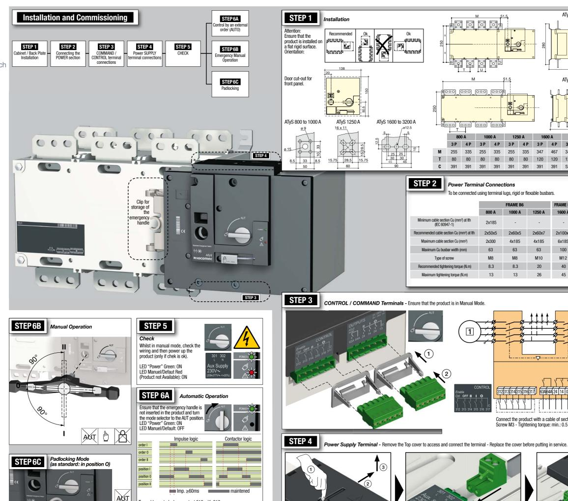
To enable control, close contact 312 with 317. To force the product to 0 position/OFF bridge
