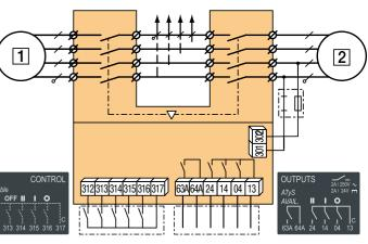
Connect the product with a cable of section of 1,5 to 2,5 mm<sup>2</sup> Screw M3 - Tightening torque: min.: 0.5 Nm - max.: 0.6 Nm
